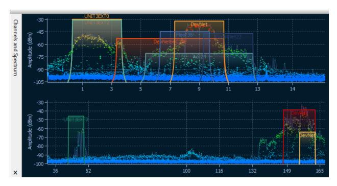
The spectrum pane is similar to the one you can see in *Chanalyzer*, a spectrum analysis application by MetaGeek that comes with Wi-Spy. By default, the **Channels and Spectrum** pane displays one or two planar spectrum graphs for single- and dual-band Wi-Spy models, respectively.
